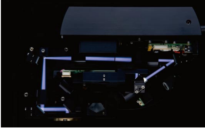
Excitation (left) and emission (right) beams in the open VivaTome unit.
