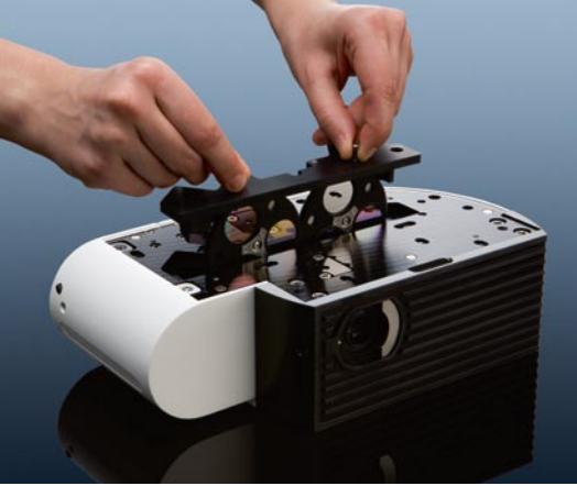
A variety of filtersets is available for VivaTome which can be easily exchanged.
