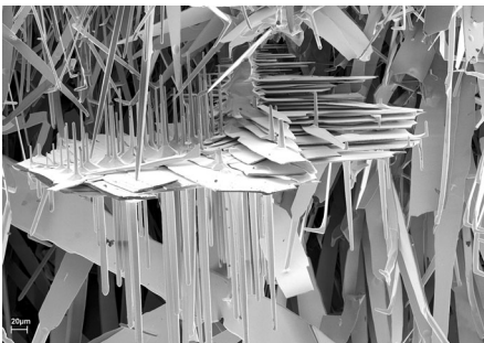
Fig. 5b: Using the HC/DoF module gives a dramatic improvement of the depth of field under the same conditions as in Fig.5a. Even with a height of 4mm, the complete sample is in focus.
