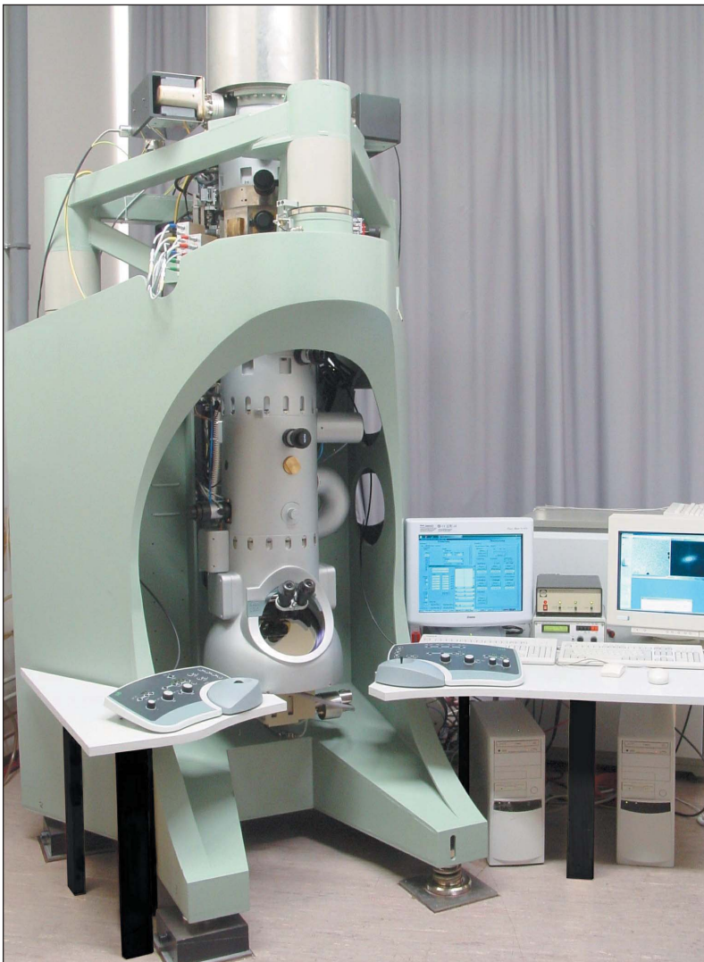
Figure 1. Carl Zeiss SMT's new sub-Angstrom UHRTEM with revolutionary column suspension concept
