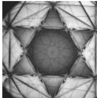
Elastic, convergent diffraction image (large angle CBED) of an aluminium specimen with [111] orientation.
