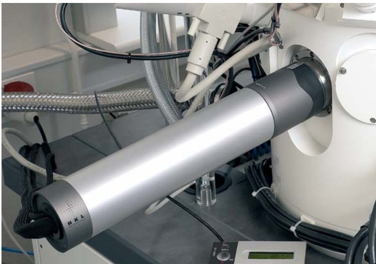
Fig. 7: SUPRA® 55VP FE-SEM with the HKL Technology Nordlys EBSD detector.
