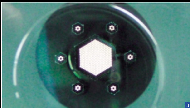
Fig. 2: PPAK fiber bundle with six small auxiliary bundles for measuring the brightness of the celestial background.
