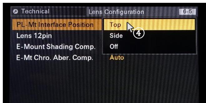
③+④ Setting up **Top** or **Side** according to the used lens contacts position of camera mount.
