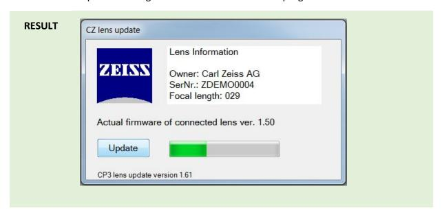
When the new firmware is transmitted on the lens successfully the installer program confirms with the following status message.
