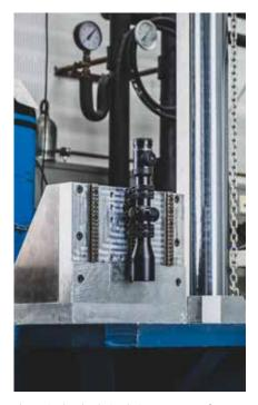
The V8 in the shock simulation test. Even after 800 shocks, the group remains unchanged.
