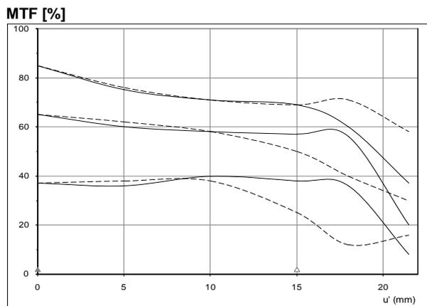
The Modulation Transfer (MTF) as a function of image height ( $u$ ) and slit orientation (sagittal, tangential) has been measured with white light at spatial frequencies of  $R = 10, 20$  and  $40$  cycles/mm. The MTF charts are valid for the ZF, ZF-I version and for white light.
