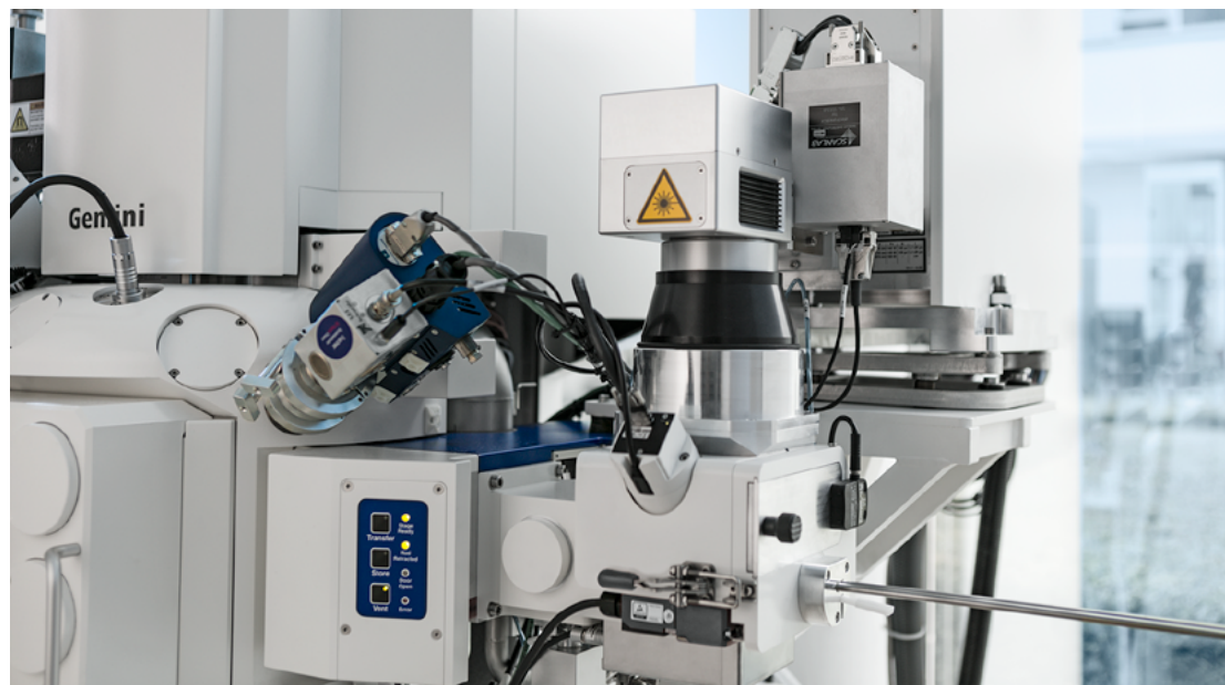
Crossbeam 350 laser. The femtosecond laser is mounted onto the airlock, thus avoiding chamber contamination during laser machining.
