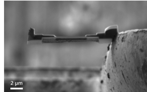
Ion-sculptor 5kV image of a lamella of poly-crystalline silicon. High imaging quality at low voltages allows precise thinning of the central region of the lamella.
